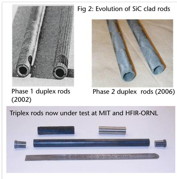
Fig 2: Evolution of SiC clad rods
