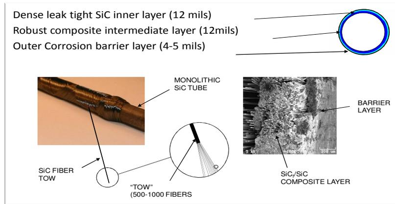
**Figure 1 – TRIPLEX<sup>TM</sup> Fuel Clad Construction**
