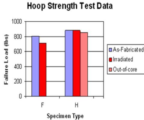
Figure 2 – MIT Reactor PWR Coolant (300 °C) Exposure Test Results
