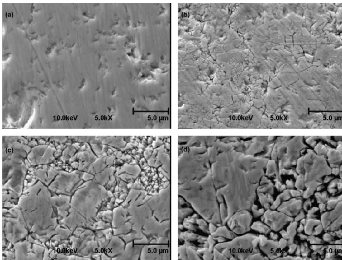
**Fig. 5.** SEM micrographs of surfaces for: (a) as-received CVD SiC; (b) after a 7-day exposure; (c) after a 14-day exposure; and (d) after a 21-day exposure.
