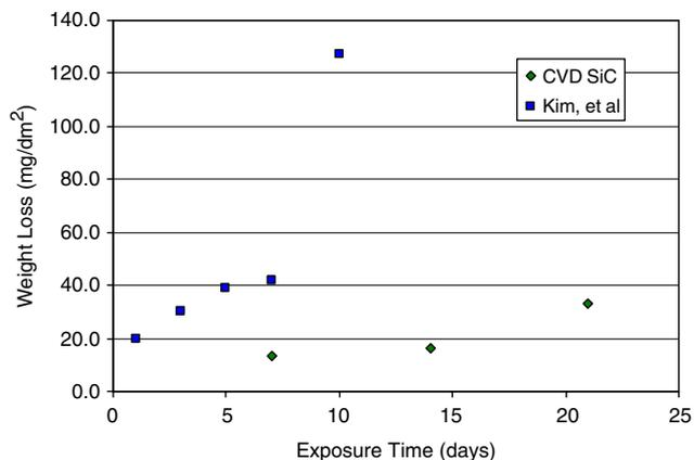
Fig. 2. Weight loss for CVD SiC after exposure to high-temperature water.
