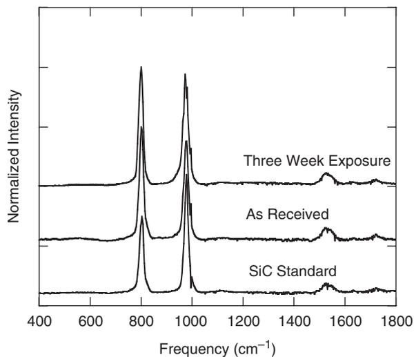
Fig. 3. Raman spectra of a stoichiometric SiC standard, the as-received CVD SiC, and the specimen surface after a 21-day exposure to 500°C water.
