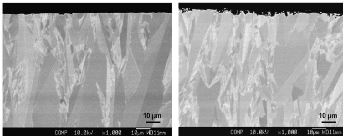
Fig. 4. SEM micrographs of fracture surfaces for as-received CVD SiC (left), and after a 21-day exposure to 500°C, 25 ppb O<sub>2</sub> supercritical water (right).
