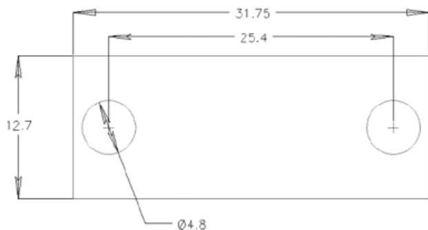
Fig. 1. SiC corrosion coupon geometry (dimensions in millimeter).
