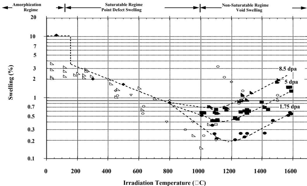
Figure 6 - Volumetric Swelling for SiC (redrawn from reference 3)
