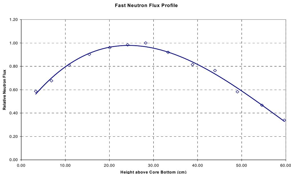
Figure 1 - Neutron Flux Profile in MITR-II Reactor
