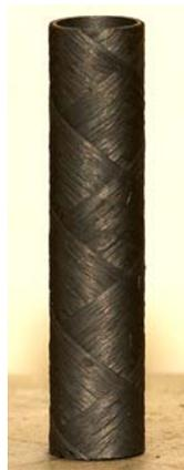
Figure 4 - Specimen F1-4 after 12 months exposure in MIT reactor
