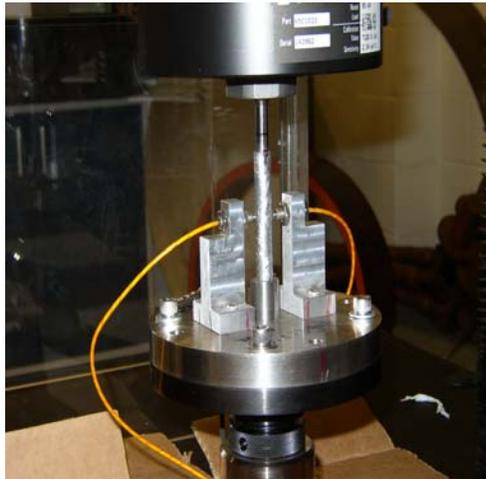
Figure 1. Test set-up showing the test specimen, the loading pistons and the proximity gages
